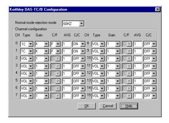
As confirmed by the Meter tab of AIO Panel, channel 0 is configured for temperature measurements and degrees F. When using a full fledged programming language such as Visual Basic, VC++ or Delphi, the DriverLINX driver will permit programmatic channel configuration, so configuration via the above screen is not necessary if performed in the code.
